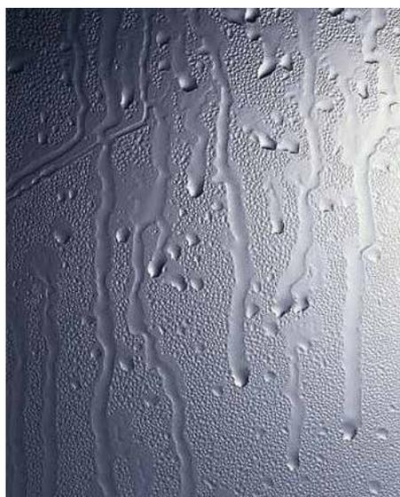
In a classroom with 20 to 30 children present at the same time, generation of water in the form of vapour can reach 1kg/h (depending on time of year). An indoor relative humidity between 35% and 65% is considered comfortable for the occupants and adequate to maintain the fabric of the buildings. Below 30%, the air becomes too dry; above 70%, the air becomes too humid.
