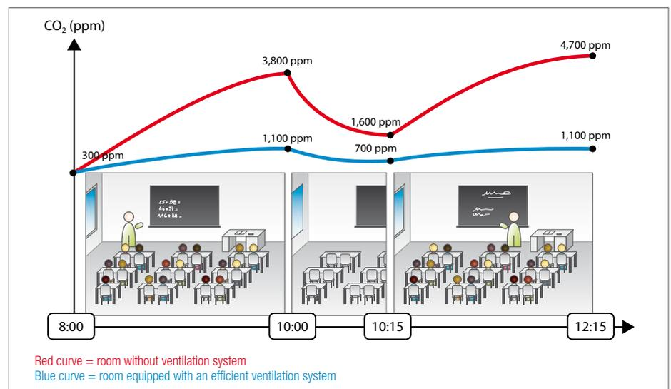
opening windows between classes is not enough to bring it down to acceptable levels. With an efficient ventilation system, CO<sub>2</sub> concentration is maintained at a level
