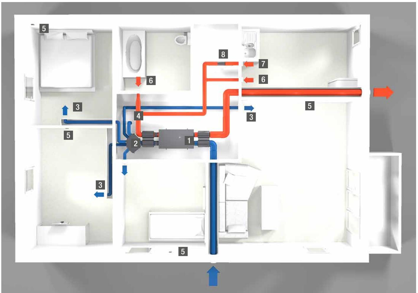
The DXR system is comprised of a heat recovery unit (DXR Unit) connected to exhaust units and to a distribution box (DXR Hub) which controls the supplied airflows. The counter-flow heat exchanger, integrated into the main unit, ensures the recovery and transfer of most of the energy from the exhaust air to the supply air, thus limiting the energy required to heat the fresh air.
